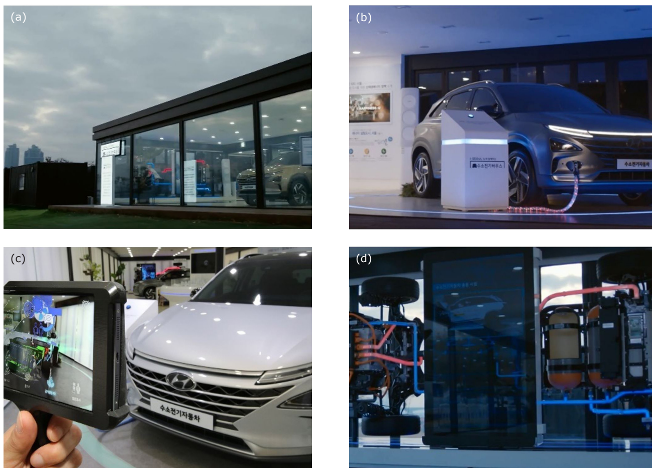
Fig. 13. Hydrogen Electric House project using Hyundai's FCEVs which supply electricity, heat and water for the House: (a) a photo of the Hydrogen Electric House; (b) an FCEV generating electricity; (c) the internal structure of an FCEV by an augmented reality technique; (d) a photo showing fuel cell components and systems of an FCEV
