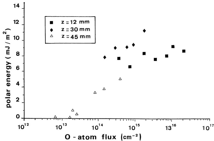
**Figure 3.** The variation in polar energy of polypropylene with the surface O atom flux ( $\text{cm}^{-2}$ ).  $z$  is the position of the substrate in the plasma reactor of figure 1.
