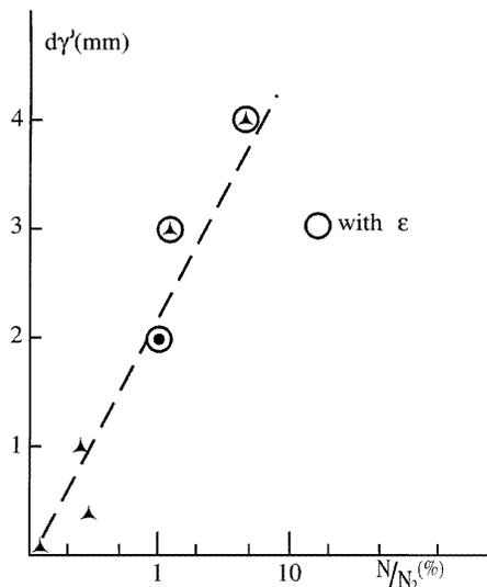
Figure 8. The variations in  $\gamma'$  layer thickness with the percentage degree of dissociation of  $N_2$  in an Ar- $N_2$  microwave post-discharge plasma.
