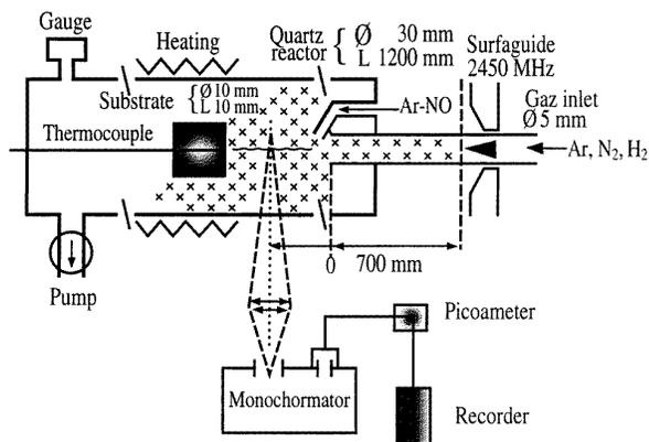
**Figure 6.** The microwave post-discharge reactor for metal-surface nitriding. The discharge tube diameter is 0.4 cm; the reactor diameter is 3 cm and its length is 100 cm.
