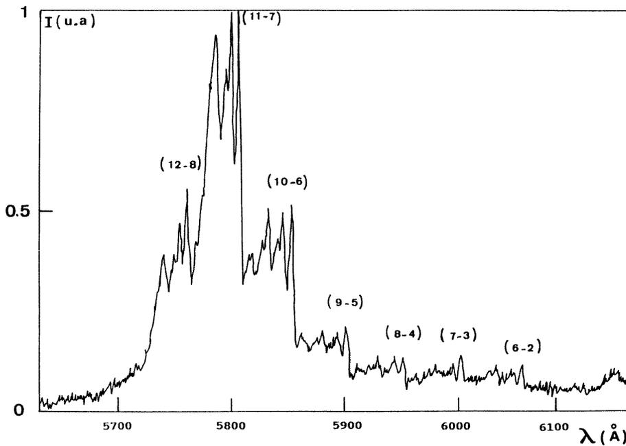
Figure 7. The intensity of the first positive system of  $N_2$  in a flowing post-discharge  $N_2$  plasma.
