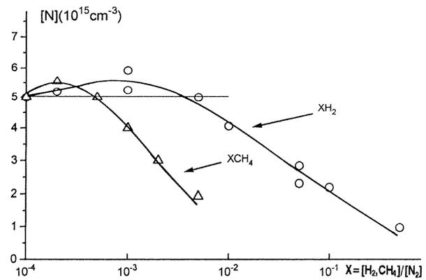
Figure 9. The N atom density versus the  $H_2:N_2$  and  $CH_4:N_2$  density ratios.
