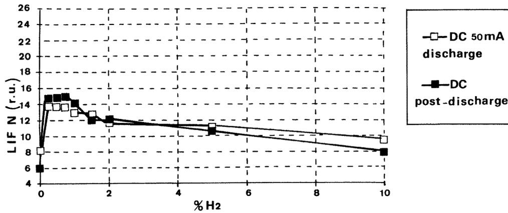
**Figure 10.** The LIF signal intensity of N atoms versus the percentage of H<sub>2</sub> in a N<sub>2</sub>-H<sub>2</sub> DC discharge and under DC and HF post-discharge conditions.
