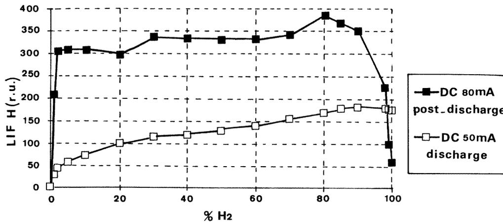
**Figure 11.** The LIF signal intensity of H atoms versus the percentage of H<sub>2</sub> in a N<sub>2</sub>-H<sub>2</sub> DC discharge and under DC and HF post-discharge conditions.
