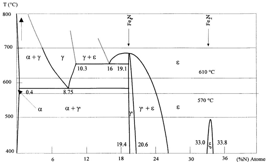
**Figure 4.** The Fe-N phase diagram.
