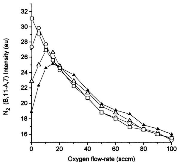
**Figure 14.** The relative intensity  $I_{\text{N}_2}$  (B,11–A,7) (proportional to  $[\text{N}]^2$ , see reaction (2)) versus the O<sub>2</sub> flow rate in a N<sub>2</sub>–O<sub>2</sub> microwave flowing post-discharge plasma at 4 Torr and 2 l min<sup>−1</sup> in a borosilicate tube of diameter 1.9 cm. The post-discharge distance was 20 cm. Tube treatment times in the N<sub>2</sub> post-discharge plasma were (□),  $t = 0$ ; (○),  $t = 40$  min; (△),  $t = 100$  min; and (▲),  $t = 460$  min.
