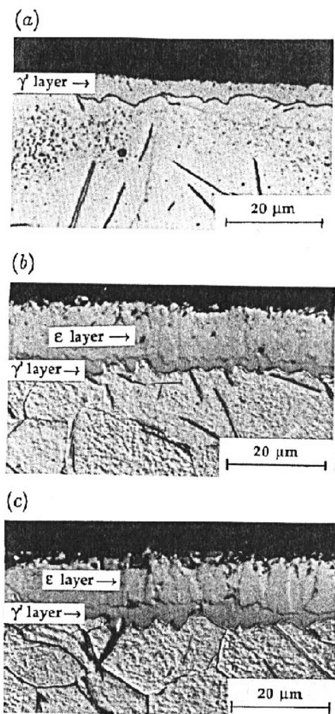
**Figure 13.** A micrograph of pure iron nitrided by a 4 h treatment in an Ar–N<sub>2</sub>–H<sub>2</sub> post-discharge plasma, with discharge parameters as in figure 12: (a)  $x = [\text{H}_2]/[\text{N}_2] = 0$ , (b)  $x = 5 \times 10^{-3}$  and (c)  $x = 5 \times 10^{-2}$ .
