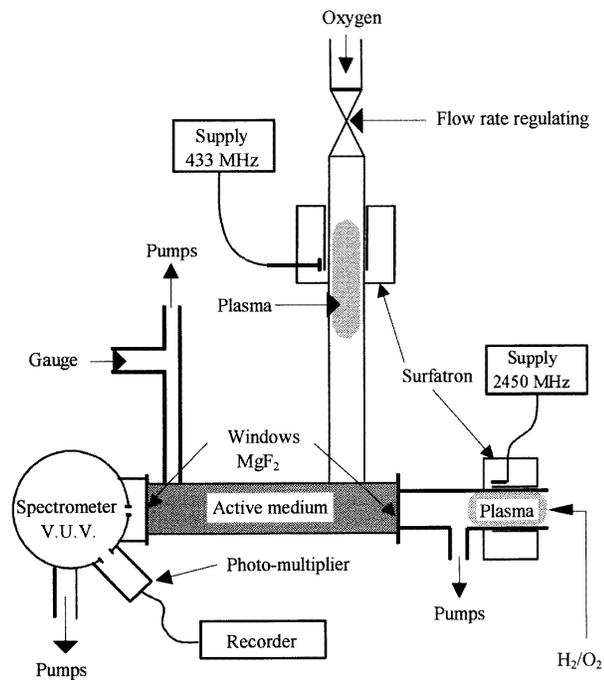
**Figure 2.** The experimental set-up for measurement of the oxygen atom density by VUV optical absorption in a microwave flowing post-discharge reactor.
