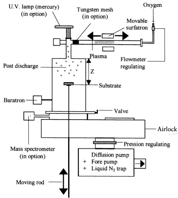
**Figure 1.** The microwave post-discharge reactor for treatment of polypropylene.
