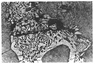
Sample  $5 \times 800$ . An area of tin-rich eutectoid (u\delta) in a copperrich matrix. N. B. Two phases are visible in the eutectoid, which is much harder than the matrix, and may have formed at the top of the casting because deliberate late additions of tin caused a higher local tin content. There is also a trace of silver present (detected by electron microanalysis).
