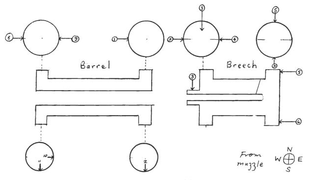
FIG. 1.-Diagram to show sampling of the cannon.
