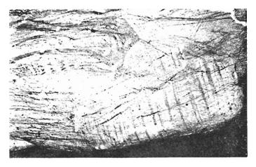
Sample  $3 \times 100$ . Quite large grains with a varied and complex strain patterns often resembling a flow pattern superimposed on fine initial slip bands.
