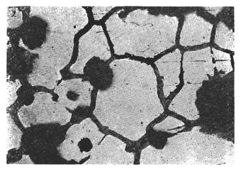
Sample 10  $\times$  100. Large equiaxed grains, without slip bands, surrounded by a thick intergranular network of slaggy material (according to electron microanalysis, mostly copper oxide Cu<sub>2</sub>O).
