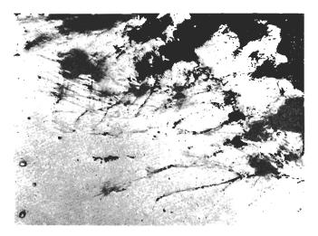
Sample  $6 \times 100$  (unetched). Note light-grey inclusions of hightin phase, and microcracks.
