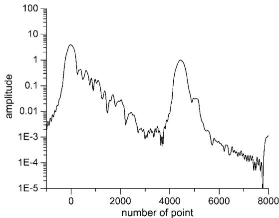
**Figure 13.** Filtering result deriving from cross-correlation result for  $c = 0.67 \text{ m}^{-1}$  and target at 5 m depth (log scale for amplitude).
