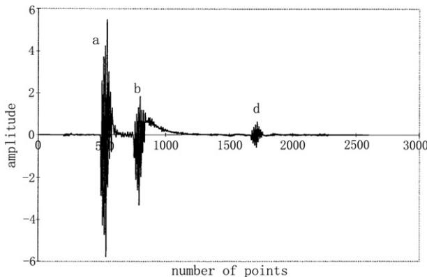
**Figure 10.** Experimental profile of cross-correlation result for  $c = 0.67 \text{ m}^{-1}$  and target at a 5 m depth.
