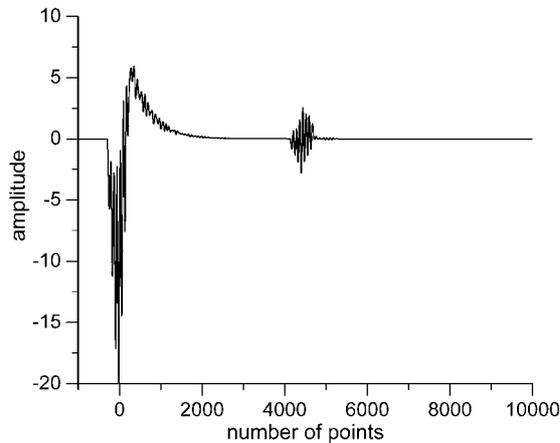
**Figure 5.** Cross-correlation result for  $c = 0.67 \text{ m}^{-1}$  and a 5 m deep target.
