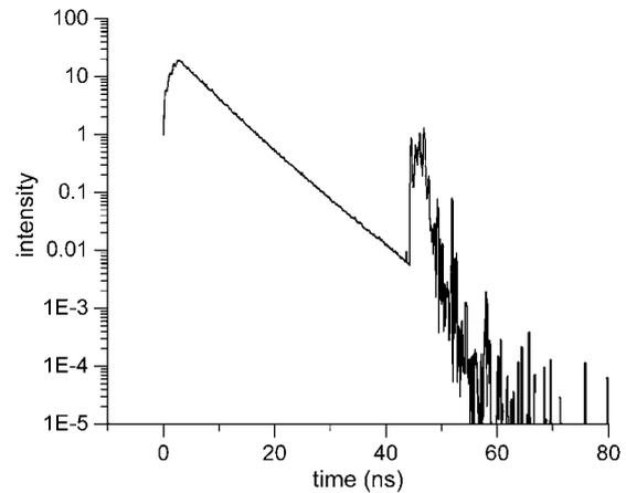
**Figure 12.** Return signal from a 5 m deep underwater target for  $c = 0.67 \text{ m}^{-1}$  (log scale for intensity).
