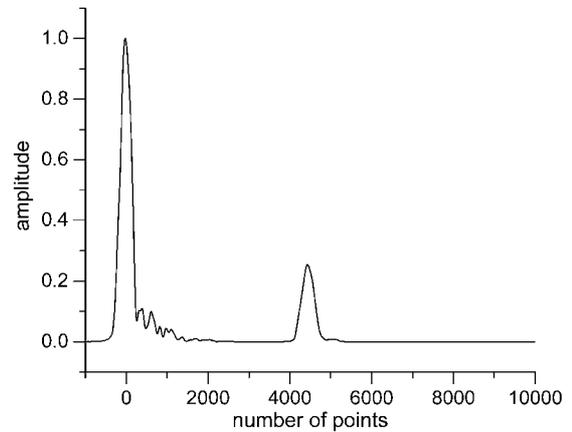
**Figure 7.** Filtering result deriving from cross-correlation result for  $c = 0.67 \text{ m}^{-1}$  and target at 5 m depth.
