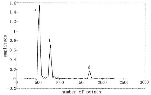
**Figure 11.** Experimental profile of filtering result for  $c = 0.67 \text{ m}^{-1}$  and target at a 5 m depth.
