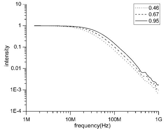
**Figure 2.** Backscattering frequency responses for  $c = 0.46, 0.67, 0.95 \text{ m}^{-1}$  (log-log scale).
