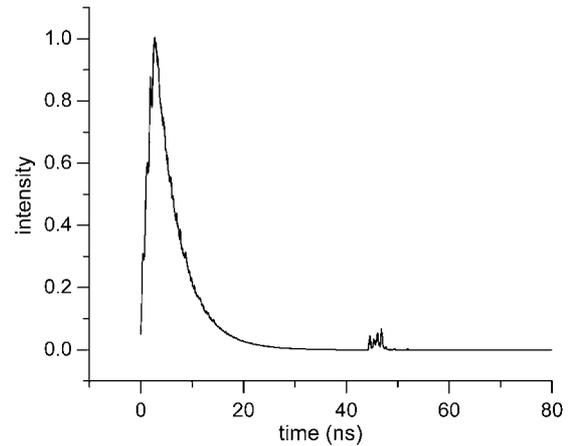
**Figure 3.** Return signal from a 5 m deep underwater target for  $c = 0.67 \text{ m}^{-1}$ .
