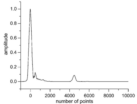
**Figure 8.** Filtering result deriving from cross-correlation result for  $c = 0.85 \text{ m}^{-1}$  and target at 5 m depth.
