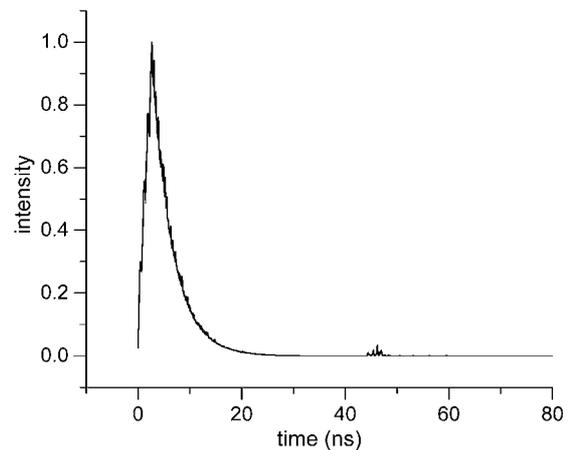
**Figure 4.** Return signal from a 5 m deep underwater target for  $c = 0.85 \text{ m}^{-1}$ .
