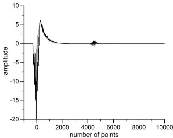
**Figure 6.** Cross-correlation result for  $c = 0.85 \text{ m}^{-1}$  and a 5 m deep target.
