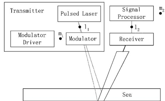
**Figure 1.** Block diagram of a modulated pulse bathymetric LIDAR system.
