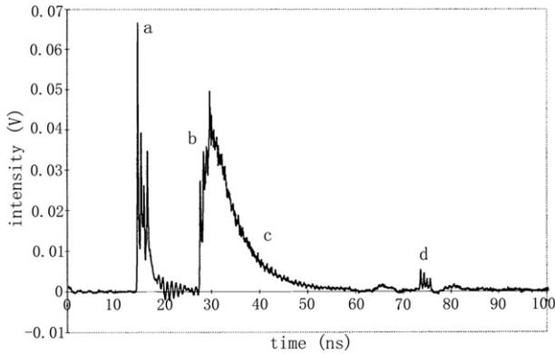
**Figure 9.** Experimental profile of backscattered signal from a 5 m deep underwater target for  $c = 0.67 \text{ m}^{-1}$ .
