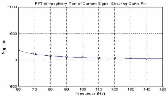
Figure -11. Curve fitting for the imaginary component of the fault current
