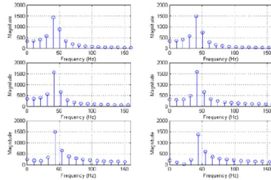
Figure-14. Obtained current block samples of the continuous fault current
