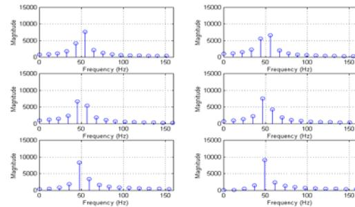
**Figure-8.** Obtained current block samples of the continuous fault current
