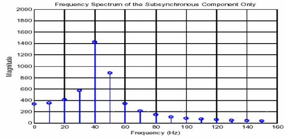
Figure-12: Magnitude correction component of the developed fault current
