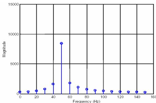
**Figure-6.** Magnitude correction component of the developed fault current
