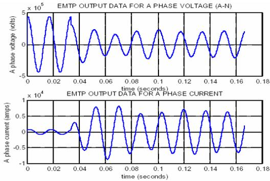
Figure- 9. Fault observed at line phase A.
