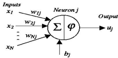
**Figure-1.** Information processing in a neural network unit.
