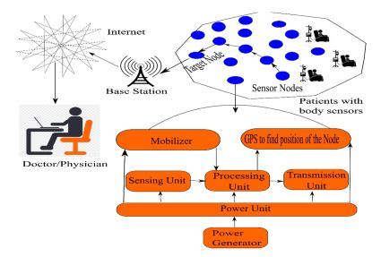
Figure 1. Sensor node architecture with application in e-healthcare.
