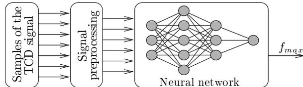
Fig. 3. General idea of the neural network based  $f_{max}$  estimation.
