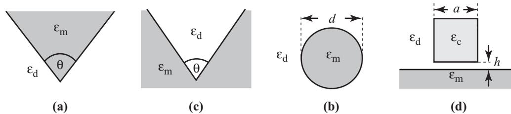
**Figure 1.** Schematics of plasmon supporting waveguides under investigation: (a) metal wedge [6, 7]; (b) groove in metal plane [9, 10]; (c) metal cylinder [3]; and (d) hybrid of dielectric and plasmon waveguides [12].
