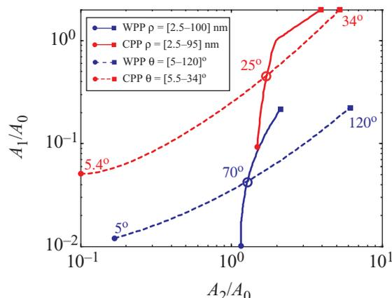
**Figure B.2.** Comparison of effective mode area,  $A_1$  and  $A_2$  in CPP and WPP waveguides parameterized by the tip radius,  $\rho$  (solid lines). Broken lines show the same comparison for  $\rho = 10$  nm parameterized by the sidewall angle,  $\theta$ .
