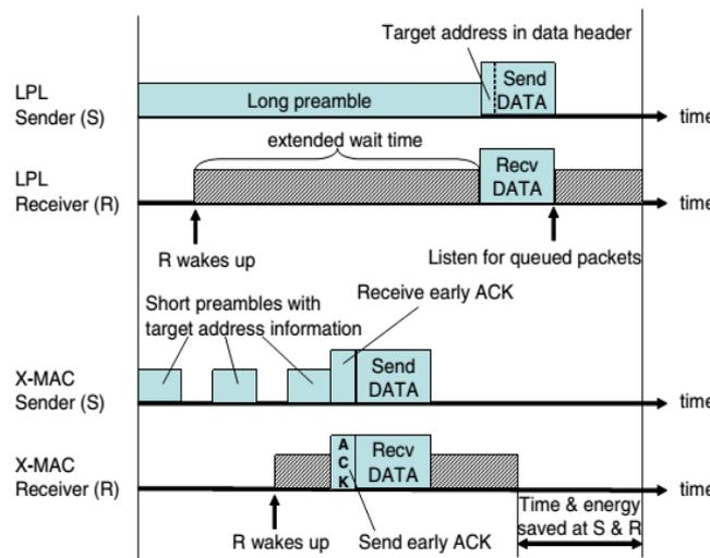
Figure 7. Comparison of the timelines between LPL's extended preamble and X-MAC's short preamble approach
