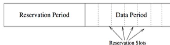
Figure 8. General frame structure for TDMA-based MAC protocols
