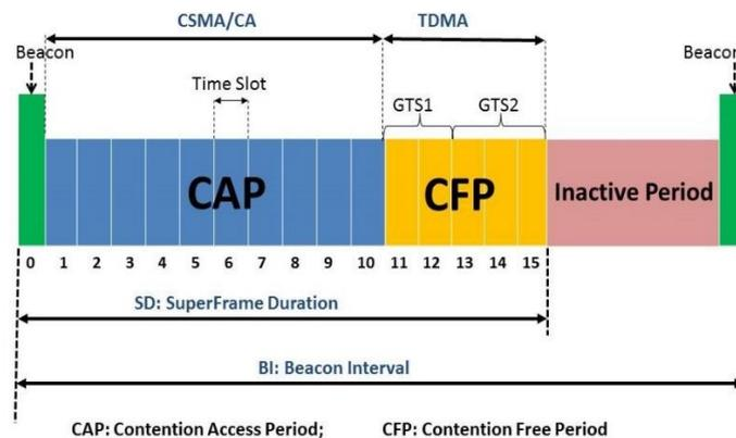
Figure 10. Super-Frame structure of IEEE 802.15.4
