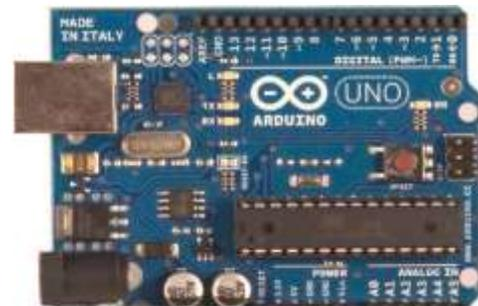
**Fig 3.3 Arduino Atmega328 Controller**
