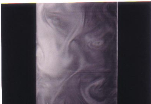
Figure 6. LIF picture showing unsteady-laminar convection. Tube diameter = 19.85 mm; Tube length = 300 mm; concentration difference = 0.025 g/cc.
