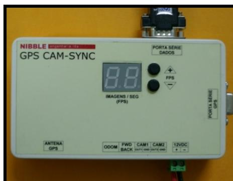
The navigation data, stored in a flash memory once per second, is composed by WGS84 latitude and longitude, height, car velocity and time in UTC (Universal Time Coordinated) format. The instantaneous vehicle heading is derived from the GPS trajectory as it is allowed by its smoothness. Horizontal accuracy, as indicated by the manufacturer, is around two meters which is sufficient for many kinds of road infrastructure inventory.
