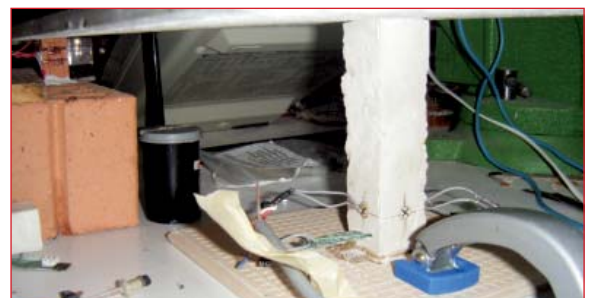
Fig. 6: Thick film sensors embedded in plaster column to measure stability.
