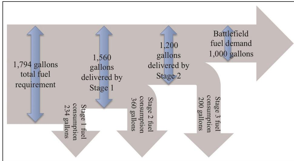
**Figure 1.** Illustration of fuel consumption in three-stage supply chain from Table 1.
