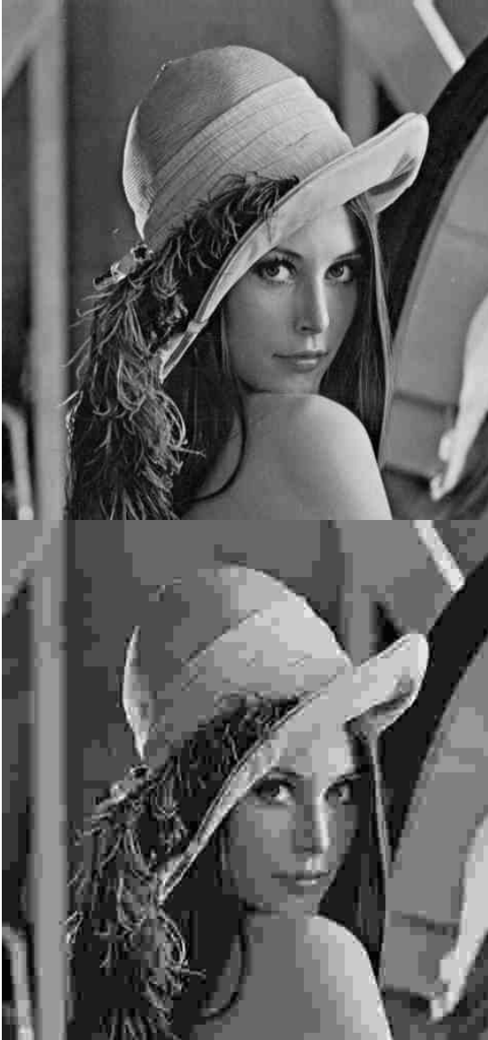
Fig. 10. Comparison of JPEG and HVS-based wavelet VQ reconstructed images: (a) JPEG, 0.458 bpp; (b) HVS-based wavelet VQ, 0.167 bpp.
