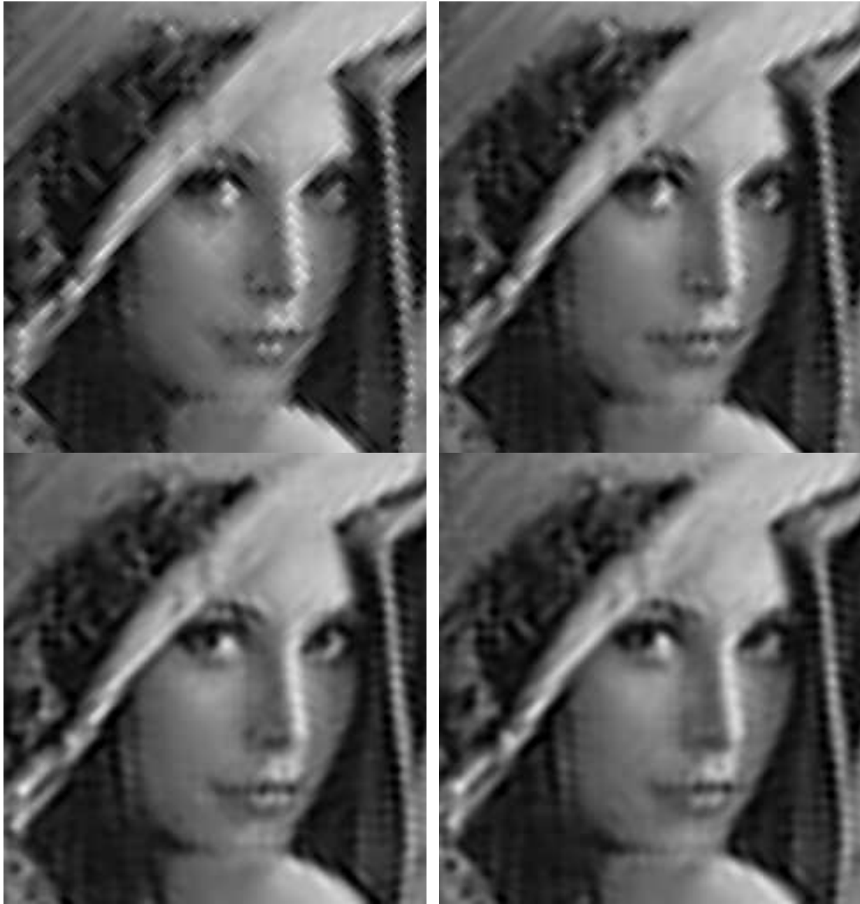
Fig. 7. HVS-based wavelet VQ reconstruction with varying filter order: (a) 4-th order filter, 0.167 bpp; (b) 6-th order filter, 0.167 bpp; (c) 10-th order filter, 0.166 bpp; (d) 12-th order filter, 0.169 bpp. Partial view, zoomed.
