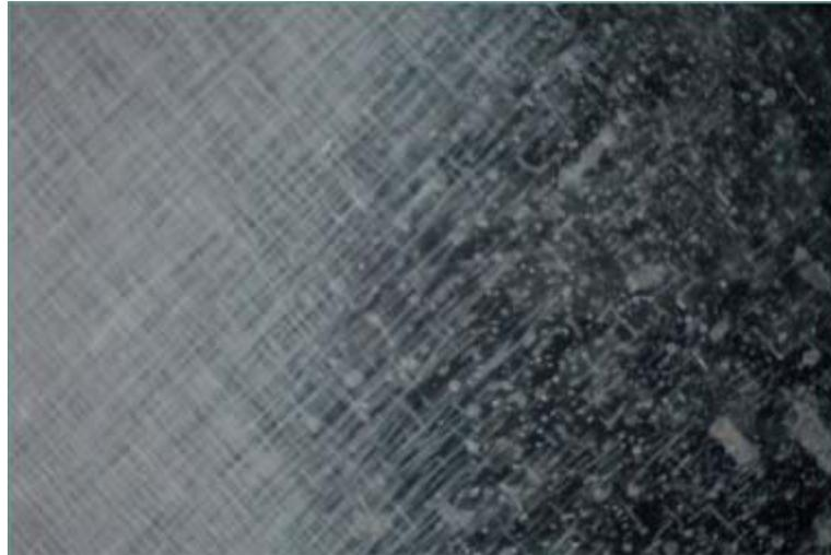
**Figure 2.** Defects in laminate after fatigue stress (16 x magnification).
