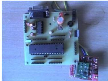
Fig.6 Photo image of working prototype model of active RFID tag
