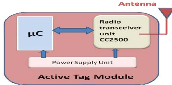
Fig.2 Block diagram of active tag module
