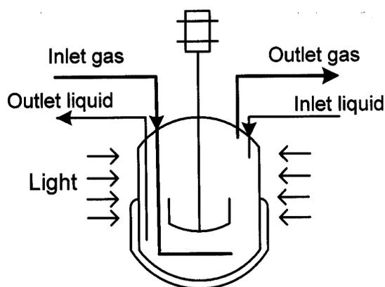
**Fig. 3. Fed-batch or continuous flow reactor.**
