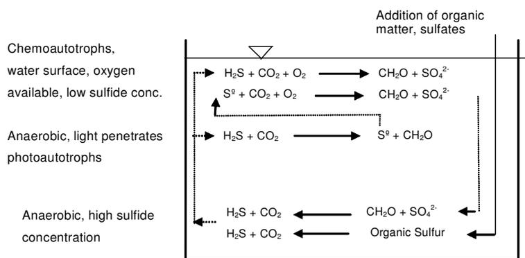
**Fig. 1. Cycling of sulfur in a sulfuretum (adapted from Anderson 1978).**
