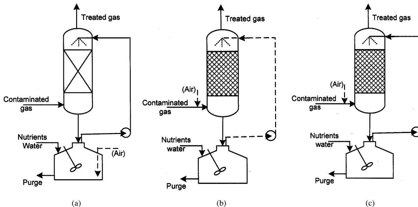
Fig. 5. Systems for removal of H<sub>2</sub>S: (a) bioscrubber; (b) biofilter; (c) biotrickling filter.
