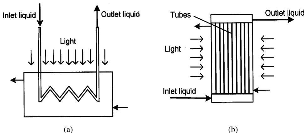
**Fig. 4. Phototube reactors: (a) horizontal; (b) vertical.**
