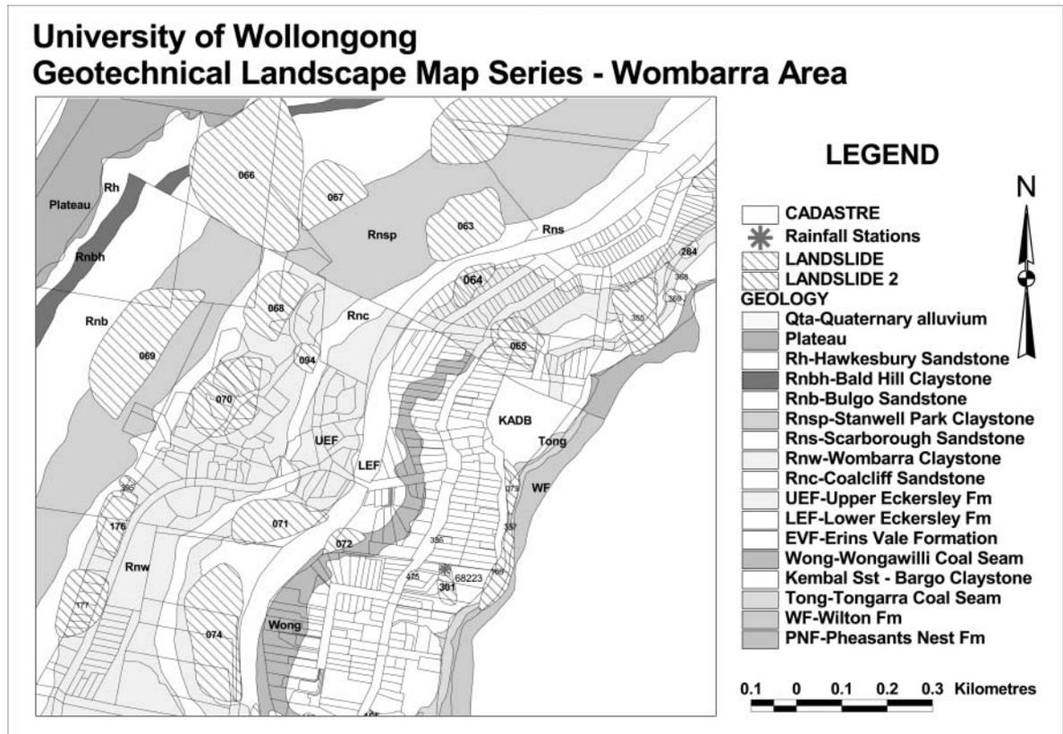
**Fig. 2.** A segment of the Geotechnical Landscape Map Series. Geology, Landslides and Cadastre Themes are shown. Each known landslide is labelled with its unique three digit Site Reference Code. Site 064 is discussed in the text.
