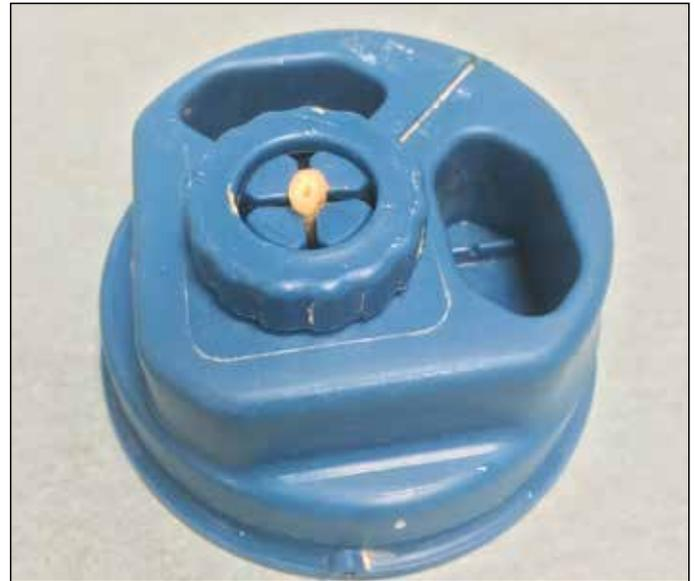
Figure 1. Sample mounted on a Protrain device (Simit, Mantua, Italy)
