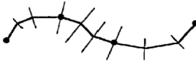
Figure 2: A stroke defined by 4 control points with intervening nodes generated by a cubic spline. The area covered by the stroke is approximated by quadrilaterals.
