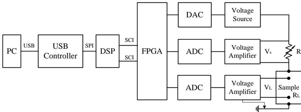
**Figure 1.** Structure of the new KHU Mark2 BIS system.
