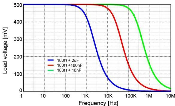
**Figure 3.** PSPICE simulation of load voltage across a parallel RC circuit (blue line:  $100\ \Omega + 2\ \mu\text{F}$ , red line:  $100\ \Omega + 100\ \text{nF}$ , green line:  $100\ \Omega + 10\ \text{nF}$ ).
