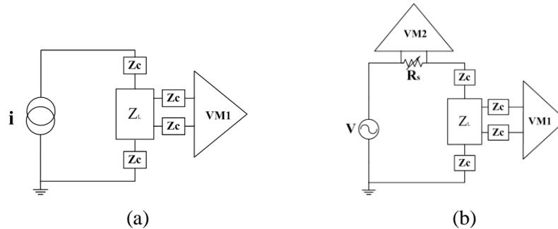
**Figure 2.** Tetra-polar electrode configuration for (a) current source and (b) voltage source. VM is a voltmeter and  $Z_C$  is a contact impedance.
