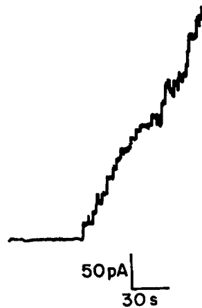
FIGURE 7. Single-channel insertion of Triton-solubilized VDAC. An asolectin membrane clamped at V = 10 mV separates solutions containing 100 mM NaCl, 10 mM MES, 0.1 mM EDTA, pH 6.0, in both compartments and in addition 40 mM \text{CaCl}_2 in the cis compartment. Just prior to the start of the record, Triton-solubilized VDAC was added to the cis compartment (final Triton concentration = 3 \times 10^{-4}\% ). Current jumps corresponding to single insertions of VDAC occur, in contrast to the multiple insertions seen when VDAC-containing vesicles are added. Neither osmotic gradients nor \text{Ca}^{++} affect the insertion process of Triton-solubilized VDAC (not shown).
