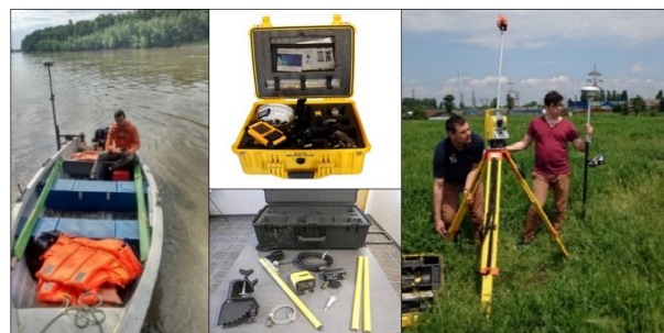
Figure 2. Left: Bathymetric depth measurements with SonarMite single-beam echosounder (SBES) (mounting method on a fiberglass rigid boat) linked to South S82-V RTK GNSS; middle: GNSS and SBES instruments and accessories; right: total station and South S82-V RTK GNSS used for topographic measurements.
