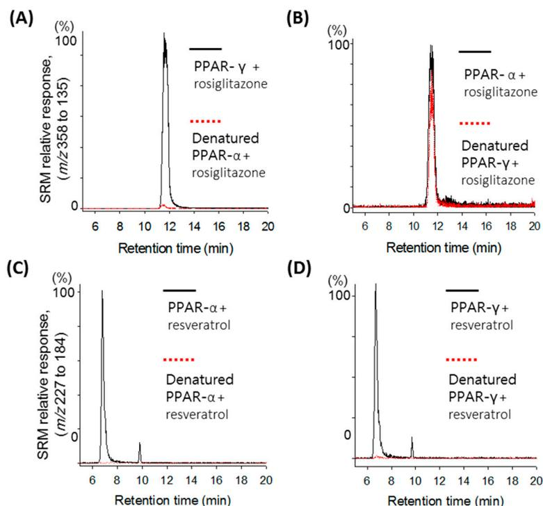
**Figure 1.** Ultrafiltration LC-MS screening of rosiglitazone and resveratrol for binding to PPAR $\gamma$  and PPAR $\alpha$ . Denatured receptor was used as a control for nonspecific binding (dotted line). Enhancement of the rosiglitazone peak compared with the control was observed upon incubation with PPAR $\gamma$  (A); but not PPAR $\alpha$  (B); whereas enhancement of the resveratrol peak was observed with both PPAR $\gamma$  (C) and PPAR $\alpha$  (D).
