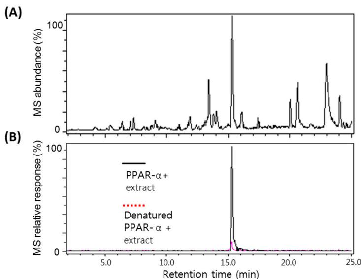
**Figure 2.** LC-MS chromatograms of an *Artemisia argyi* methanol extract (A) and detection of a positive compound (B) as a PPAR $\alpha$  ligand using ultrafiltration LC-MS. MetaboliteDetect at a setting of greater than threefold enhanced signal and less than 0.05  $m/z$  difference automatically detected a positive compound in the LC-MS chromatograms of the extract.
