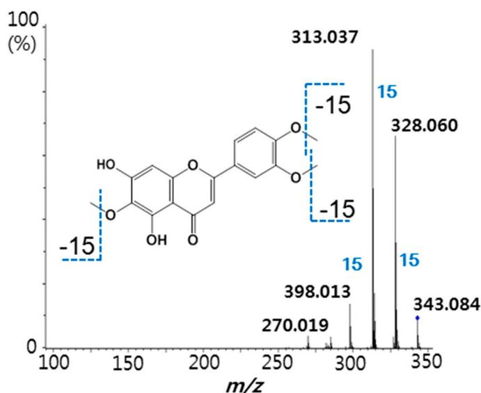
**Figure 3.** Negative ion electrospray tandem mass spectra of the deprotonated molecule of eupatilin at  $m/z$  343. Product ion mass spectra were obtained using collision-induced dissociation at 18 eV energy.
