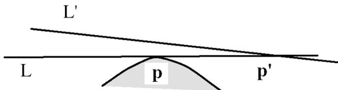
Fig.3. Only  $\mathbf{p}$  belongs to  $S_{VH}$ . Trough any other point  $\mathbf{p}'$  pass visual lines as  $L'$ .
