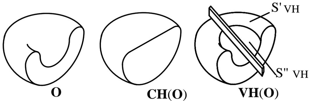
Fig.1. An object  $\mathbf{O}$ , its convex hull  $\mathbf{CH}(\mathbf{O})$  and its visual hull  $\mathbf{VH}(\mathbf{O})$
