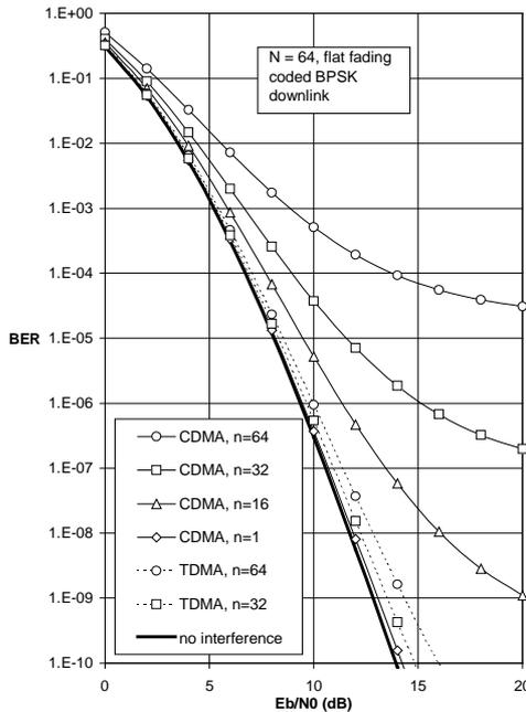
Fig. 4 : Downlink BER performance for coded transmission over flat Rayleigh fading channel
