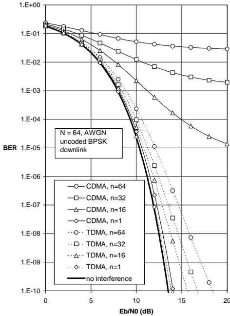
Fig. 2 : Downlink BER performance for uncoded transmission over AWGN channel
