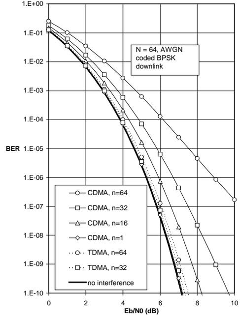
Fig. 3 : Downlink BER performance for coded transmission over AWGN channel
