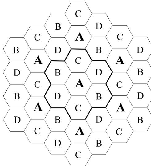
Fig. 1 : Cell structure with reuse factor of 4.
