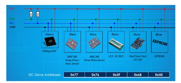
Figure 3. The implementation of  $I^2C$  bus for our home automation system.
