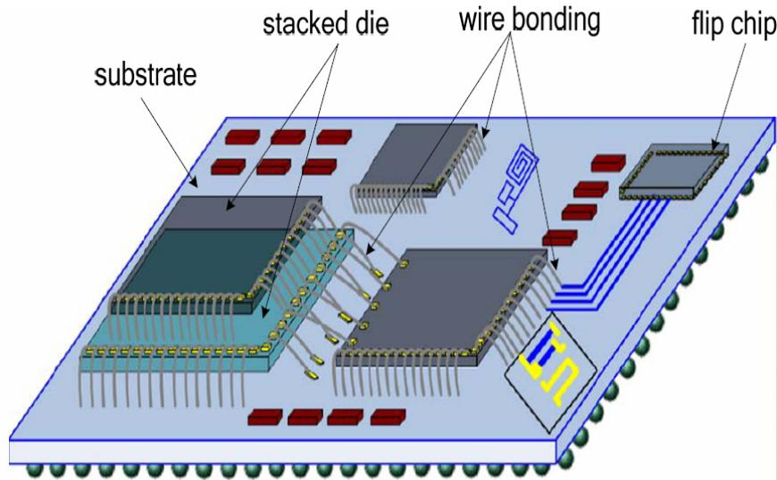
Fig. An example of IC package.
