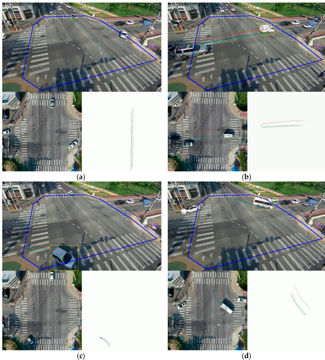
Figure 13. Results of the vehicle trajectory extraction corresponding to the different algorithms: (a) driving straight (up and down); (b) driving straight (left and right); (c) right turn; and (d) left turn.
