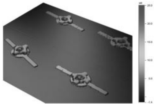
Fig. 3. 3D surface topology of a 2 × 2 mixer array measured by an optical profilometer (Veeco NT1000).
