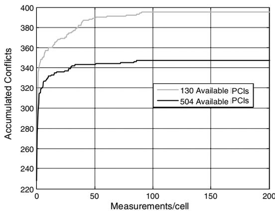
Figure 6. The maximum number of PCI is set to 130 and 504, respectively. All cells were initiated with identical PCI.
