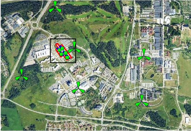
Figure 3. Aerial view of the fictitious deployment in Mjärdevi Linköping. The outer walls of the building are marked with grey (red) lines. The inner walls (facing the in-between building area) are marked with dark (blue) lines.
