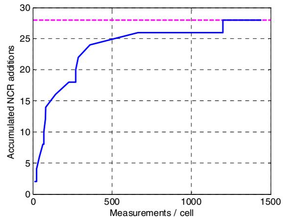
Figure 4. Neighbor cell list convergence. Accurate NCR lists are achieved after approximately 1000 measurements per cell made by mobiles in handover situations.
