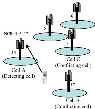
Figure 2. PCI conflict detection based on handover measurements. The mobile reports a new candidate cell with a PCI already present in the NCR list of the serving cell.
