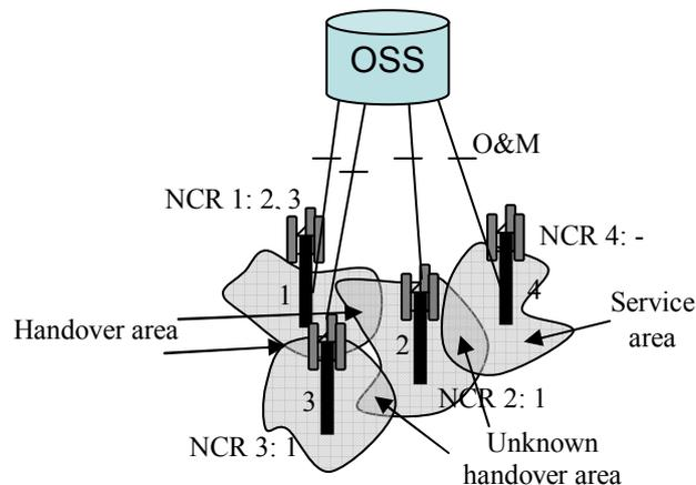
Figure 1. OSS monitors neighbor cell lists, and manages PCIs. Some cells have complete knowledge of the neighbor relations (cell 1), some cells miss neighbor relations possibly due to inaccurate models in the planning step (cell 2 and 3) and some cells are newly installed without neighbor info (cell 4).
