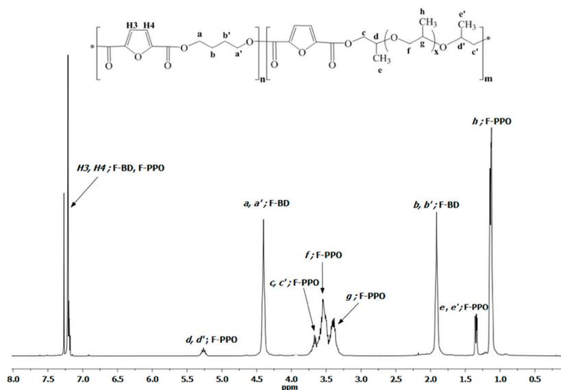
Figure 2.  $^1\text{H}$  NMR spectrum of PBF-*co*-PPOF-90/10 co-polymer in  $\text{CHCl}_3$ -*d*.
