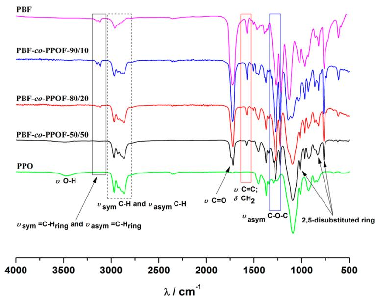
Figure 1. ATR FTIR spectra of PBF-*co*-PPOF co-polymers.
