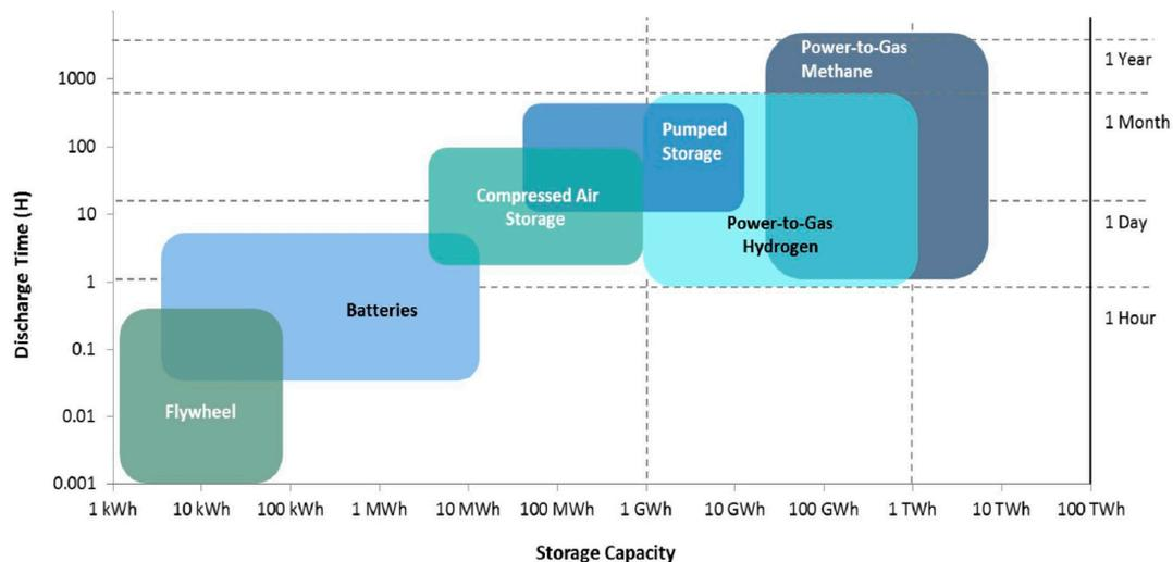
**Figure 3.** Comparison of discharge time vs capacity of energy storage technologies [24].
