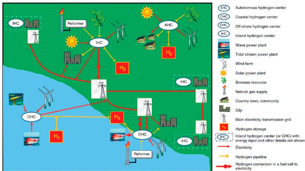
**Figure 10.** A schematic illustration of the sustainable hydrogen hierarchy proposed by Andrews and Shabani [16].
