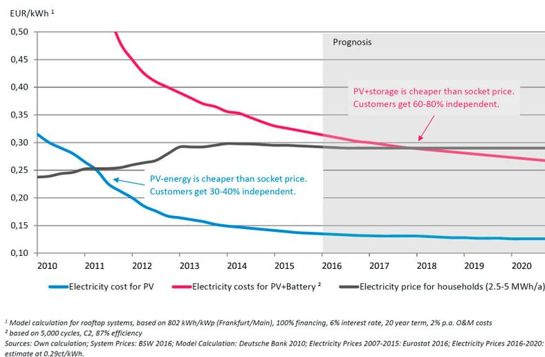
**Figure 6.** Comparison of photovoltaics (PV) grid parity and PV + battery parity in Germany [55].
