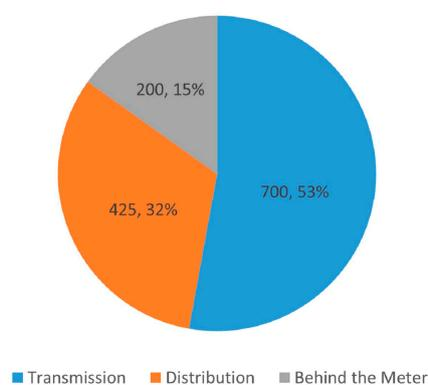
**Figure 5.** California 2020 energy storage target by network area (created from data obtained from [11]).
