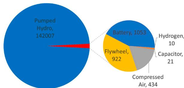
Figure 2. Global installed grid connected energy storage capacity in MW that can be used to supply electricity (created from data obtained from [7]).
