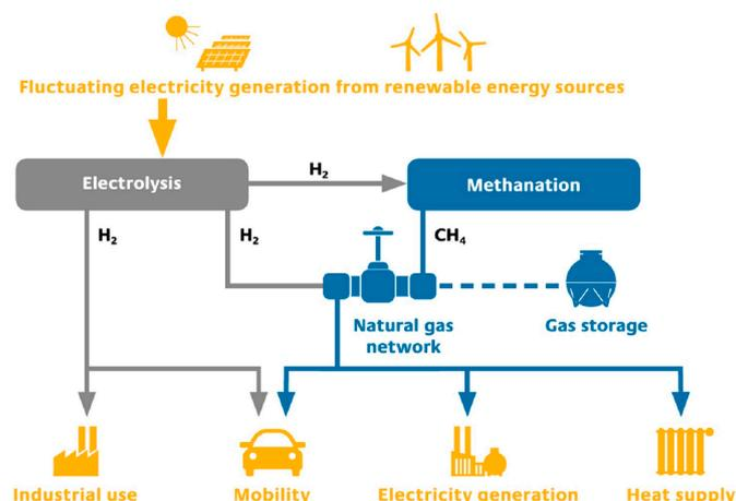
**Figure 11.** Power-to-gas (P2G) process and applications [109].
