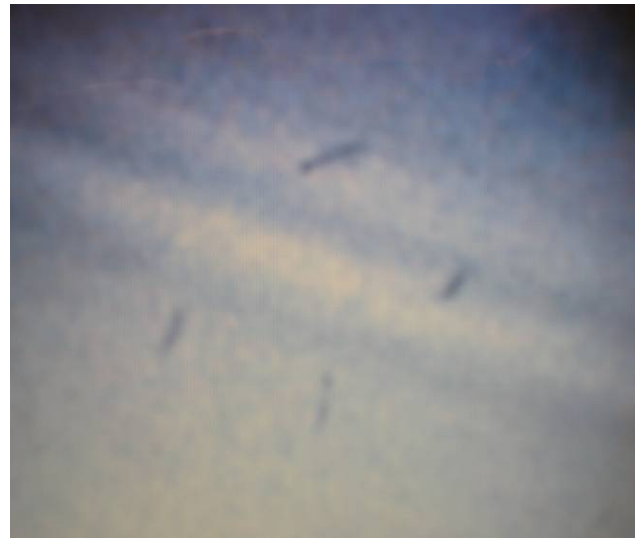
Figure 4: The defect area after 80 \mu\text{m} of tumbling. The pit is no longer visible, even at high magnifications. The dark blemishes are deposits from the tumbling media and were removed with HPR.
