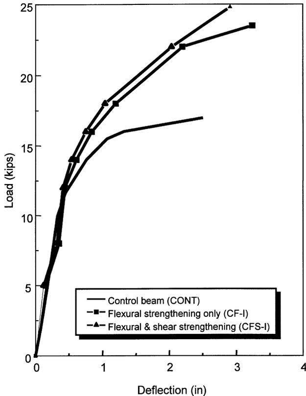
Fig. 2—Response of Group 1 strengthened beams.
