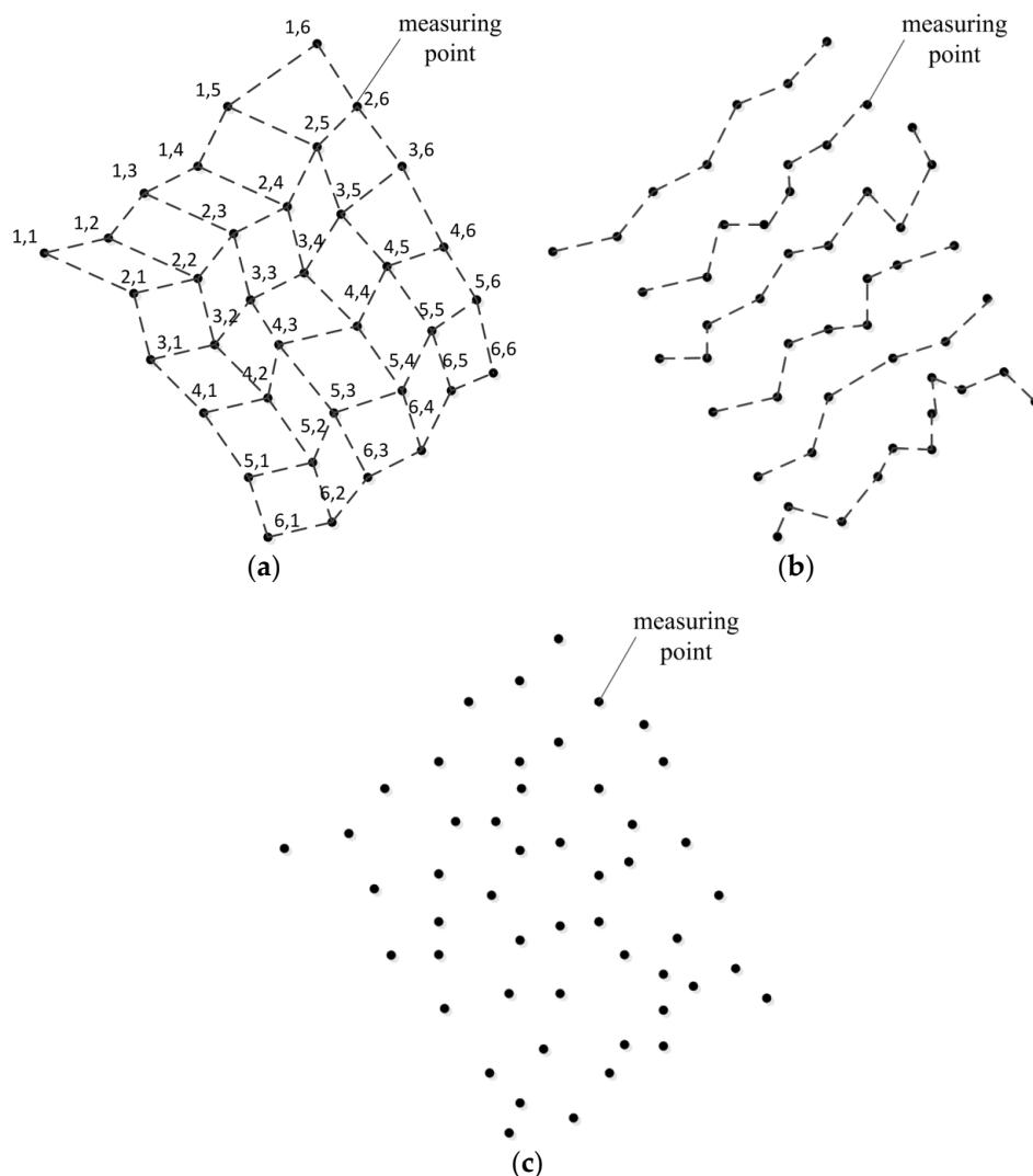
**Figure 1.** Three different kinds of distribution of data points: (a) grid data; (b) quasi-scattered data; (c) completely scattered data (quasi-scattered data is stored according to the order of measurement which is the main difference from completely scattered data).
