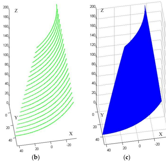
**Figure 12.** Surface fitting of a blade surface: (a) a diagram of the measurement; (b) the original grid data; (c) the randomly chosen data; (c) the fitting NURBS surface.
