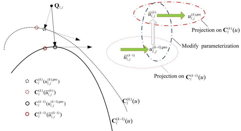
**Figure 4.** The process of iterative projection optimization during curve fitting.
