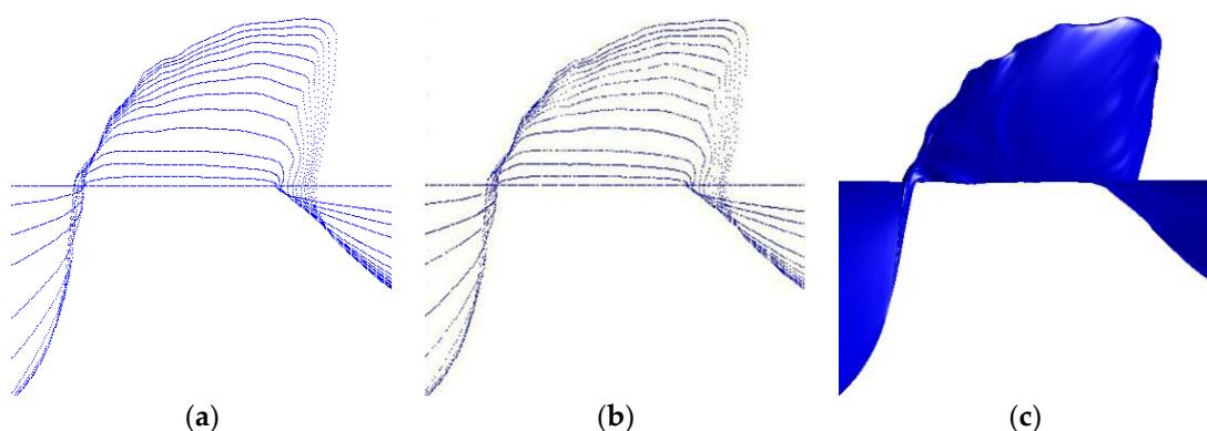
**Figure 10.** Surface fitting of a pump surface: (a) the original grid data; (b) the randomly chosen data; (c) the fitting NURBS surface.
