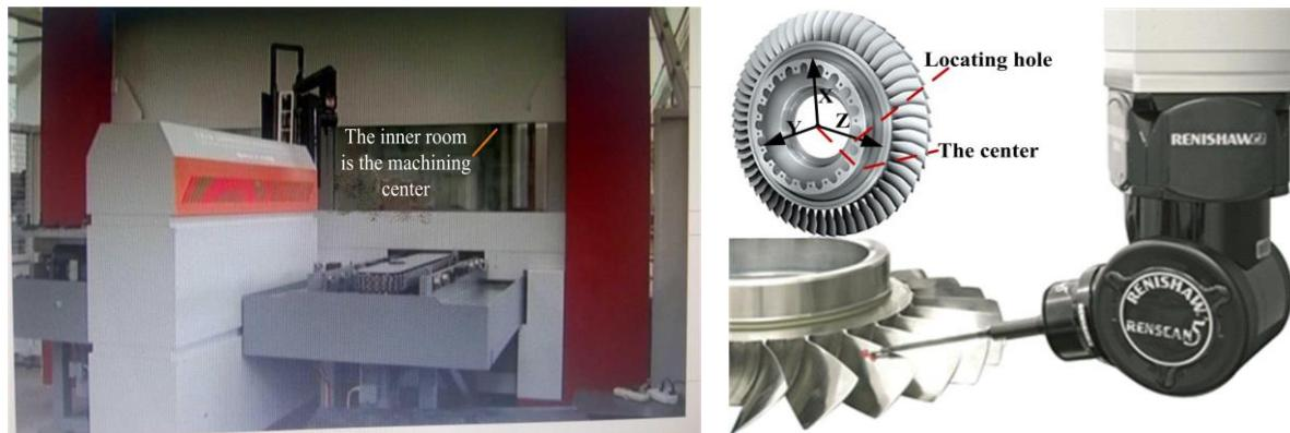
**Figure 11.** The applied coordinate measuring system: the left picture is the scene photo; and the right picture is the measurement on the workpiece.
