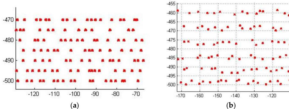
**Figure 13.** Points distribution on the  $(u, v)$  domain when sampling along  $u$ -section line: (a) the case when  $u$ -fluctuation is equal to zero; (b) the case when  $u$ -fluctuation ranges from  $-1.5$  to  $1.5$  randomly. In this picture,  $v$  direction is the horizontal direction, and  $u$  direction is the vertical direction.
