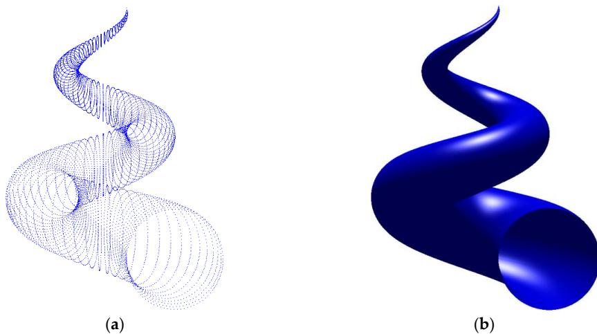
**Figure 8.** Surface fitting of a shell surface: (a) the data chosen randomly from grid data; (b) the fitting surface.
