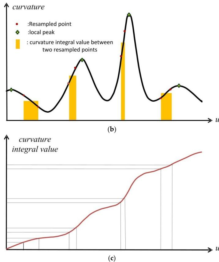
**Figure 5.** The process of resampling. (a–d) are respectively the measured data using equal parameter sampling technique, the curvature variation after GLPF, the curvature integral value, and the resampled points using the provided approach.
