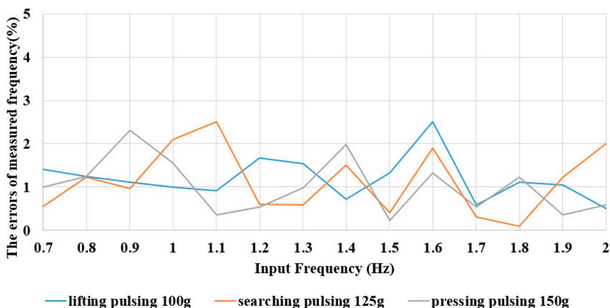
**Figure 14.** The calibrated detection system errors for 0.7 Hz–2.0 Hz frequencies.
