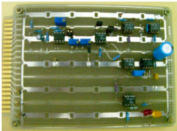
**Figure 11.** The pulse signal processor hardware.
