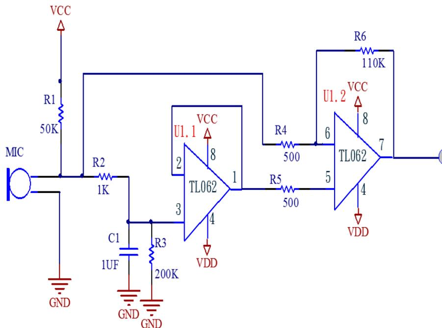
**Figure 5.** Pulse amplifying circuit.
