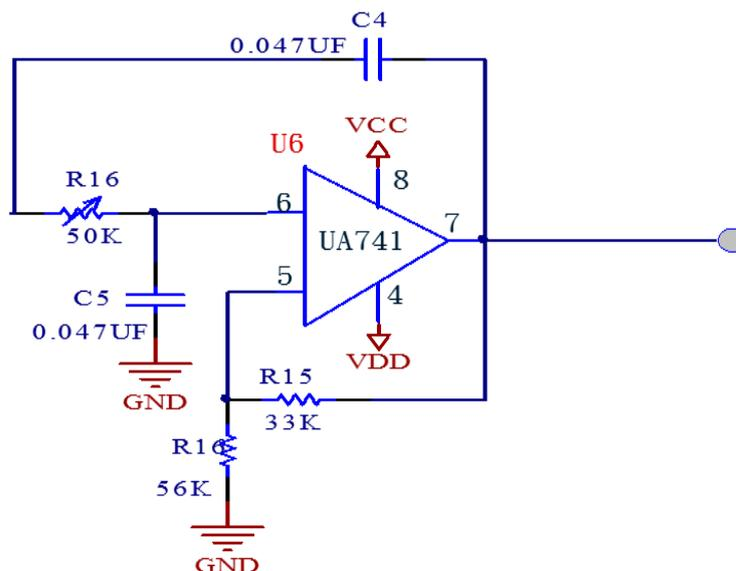
**Figure 6.** Low-pass circuit.
