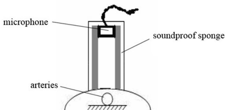
**Figure 1.** Pulse receiver.
