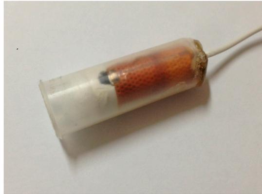
**Figure 3.** Pulse sensor.
