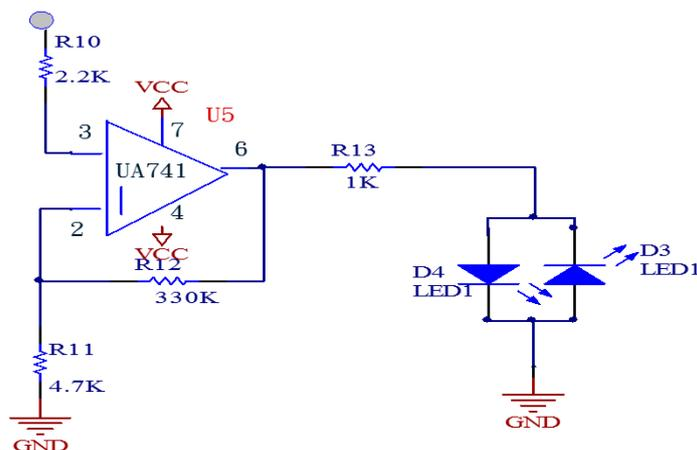
**Figure 9.** Circuit drives LED.
