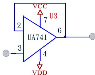
**Figure 7.** Buffer circuit.
