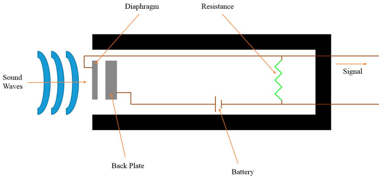
**Figure 4.** The circuit of the condenser microphone.
