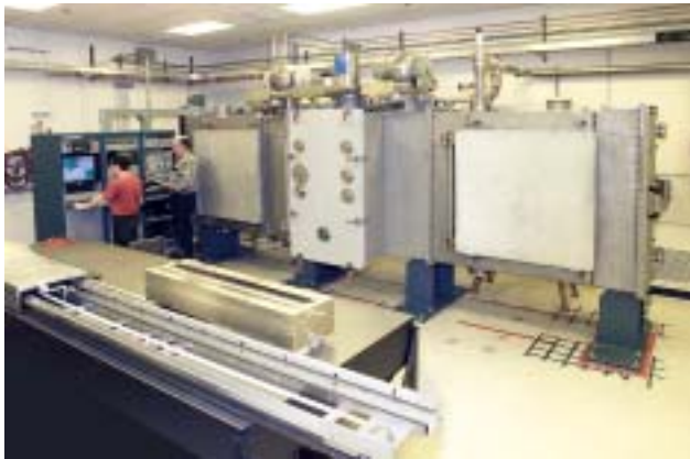
Figure 10. Photograph of the ion-beam etcher. Ion source and substrate linear motion track in foreground awaiting installation.
