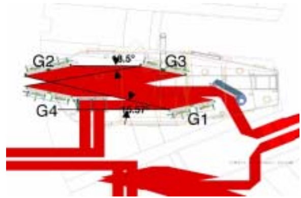
Figure 15. Compact mixed grating pulse compressor. Gratings 1&2 are 1750 gr/mm while gratings 3&4 are 1780 gr/mm. The separations and angles of incidence have been adjusted so that the output has no spatial chirp.
