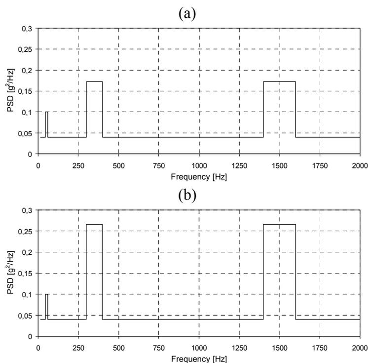
**Table 2.** Characteristics of vibration spectrum excitations for functional and endurance sections.
