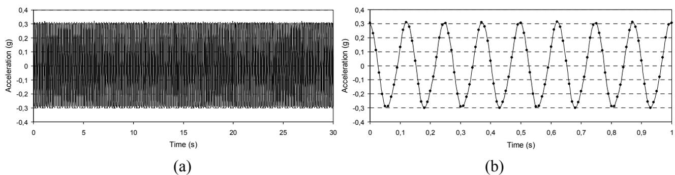
**Figure 8.** Low frequency characterization before dynamic excitation: 0.02 g amplitude, 1.5 Hz frequency, z-axis; whole acquisition (a) and detail of the wave form (b).
