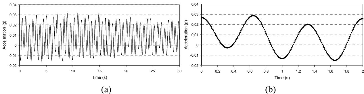
**Figure 12.** Sine sweep after dynamic excitation: 0.3 g amplitude, 0.5 Hz/s sweep ratio, y-axis. The horizontal lines correspond to the vibration level measured by the piezoelectric accelerometer used as feedback signal; (a) increasing (5–10 Hz) and (b) decreasing (10–5 Hz) frequency .
