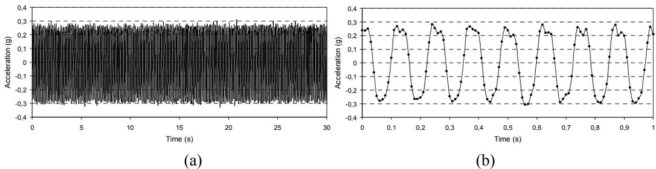
**Figure 11.** Low frequency characterization after dynamic excitation: 0.02 g amplitude, 1.5 Hz frequency, z-axis; whole acquisition (a) and detail of the wave form (b).
