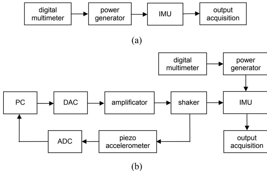
**Figure 5.** Experimental settings: (a) evaluation of static systematic and accidental errors by means of the six positions static test and the Allan variance calculation; (b) dynamic excitation step of the reliability test procedure.
