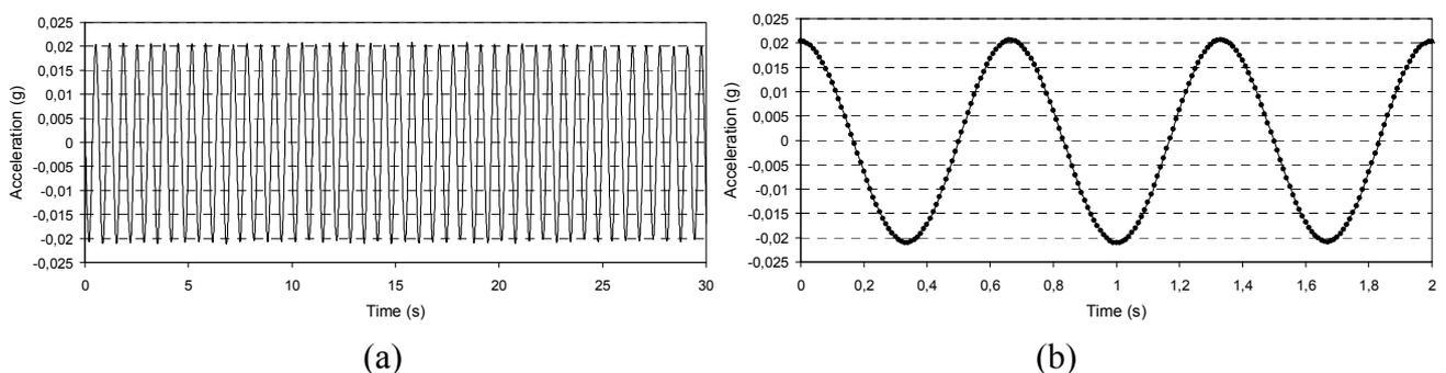
**Figure 9.** Sine sweep before dynamic excitation: 0.3 g amplitude, 0.5 Hz/s sweep ratio, y-axis. The horizontal lines correspond to the vibration level measured by the piezoelectric accelerometer used as feedback signal; increasing frequency 5–10 Hz (a) and decreasing frequency 10–5 Hz (b).
