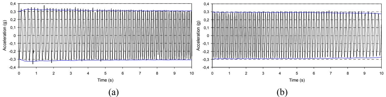
**Figure 10.** Signal stability after dynamic excitation: 0.3 g amplitude, 8 Hz frequency, x-axis; whole acquisition (a) and detail of the wave form (b).
