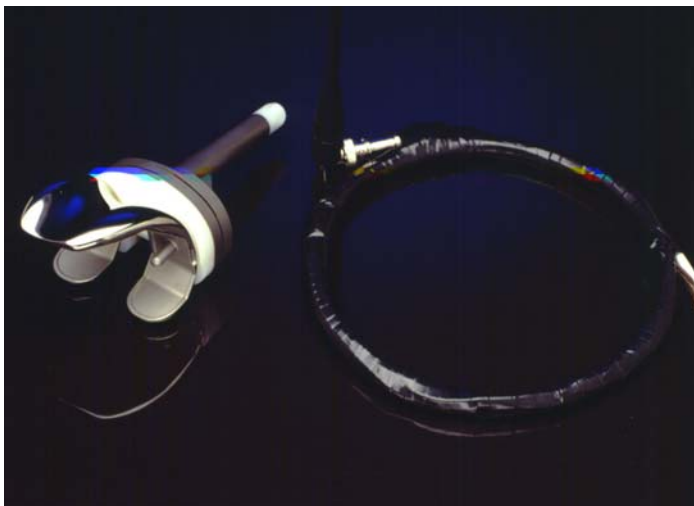
Figure 5. Remotely powered, hermetically sealed, smart total knee replacement (left) along with external powering coil and receive antenna (right). Photograph courtesy Scripps Institute.
