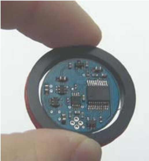
Figure 6. Switched reactance EmbedSense sensing node shown with embedded coil around periphery of circular printed circuit board module.
