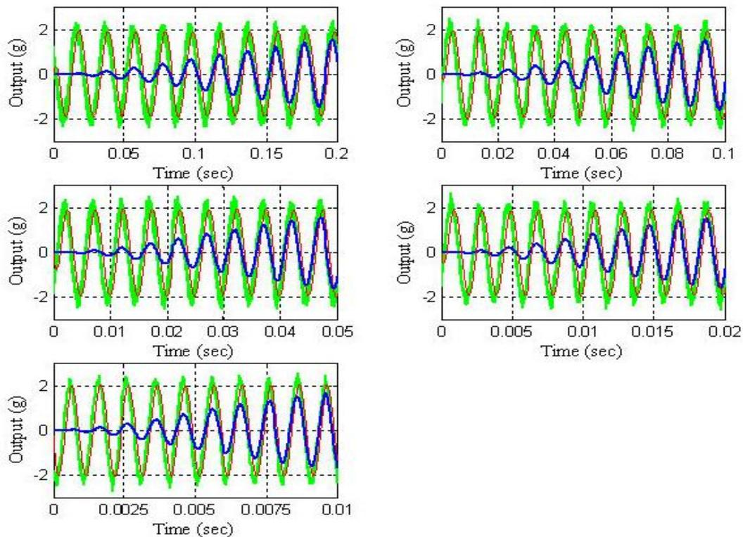
If we compare the experimental results shown in Figure 15 with the ones shown Figure 14 and analyze the results shown in Figure 17, we can see that both the *quality of the response* and the *speed of the response* of the LMS adaptive filter are better than the ones of the five 4-order band-pass digital Butterworth filters. Therefore, the best option to carry out the filtering problem discussed in this paper was to use the LMS adaptive filter.
