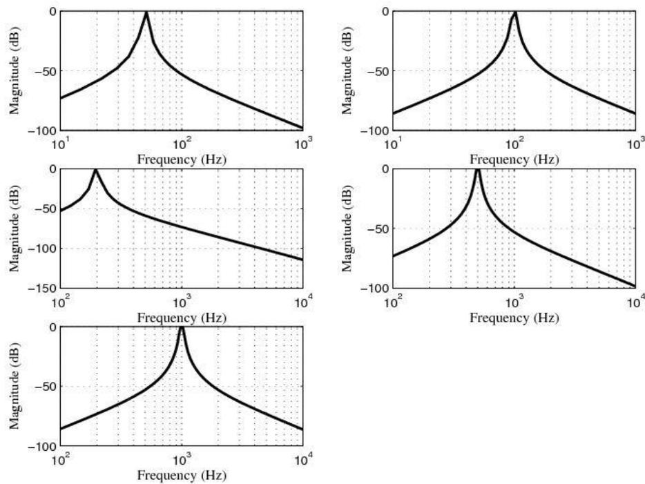
**Figure 14.** Power spectrum magnitude (dB) of the output signals after filtering by using the corresponding five 4-order band-pass digital Butterworth filters.
