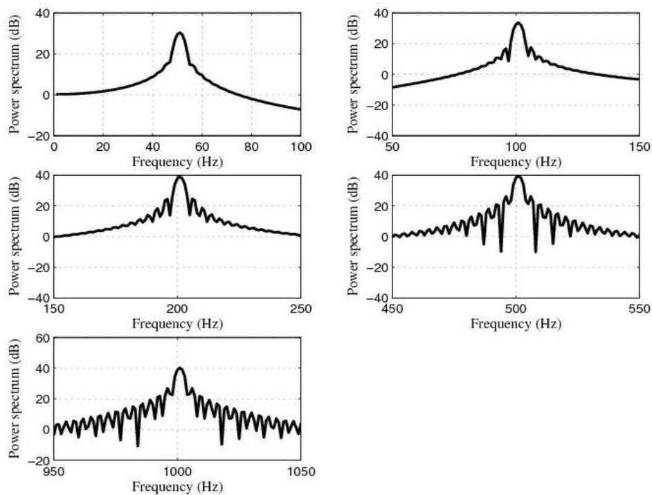
At this point, it is important to mention that the performance of the sensor system based on the five 4-order band-pass digital Butterworth filters can be considered satisfactory. However, in real automotive applications the designer does not know exactly the frequency of the relevant signal.
