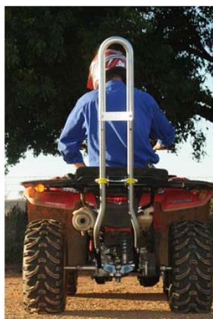
**Figure 2.** A Quadbar attached to the rear of an All-Terrain Vehicles (ATV).
