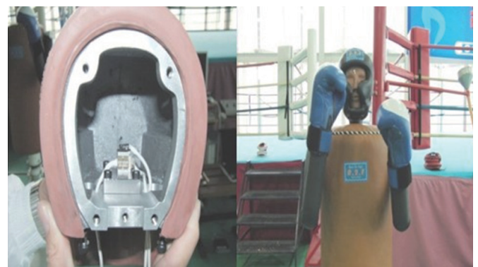
Fig. 4. Equipment for measuring punch power. Inserted three-axis acceleration sensor inside the dummy face.
