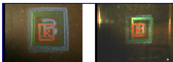
Fig. 7. Reconstructed images calculated from the microimages captured with the telecentric pickup (left movie) and with the conventional pickup (right movie). (Video file of 0.6 Mb).
