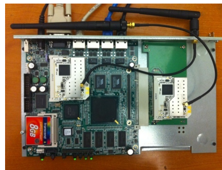
Fig. 1. The Soekris Net-5501 board.
