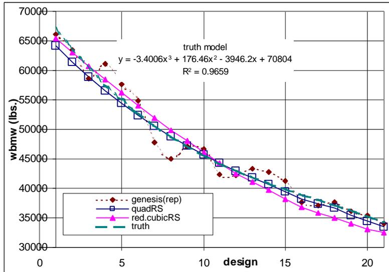
Figure 9: Comparison of correction RS approximations and GENESIS results along extreme value design line
