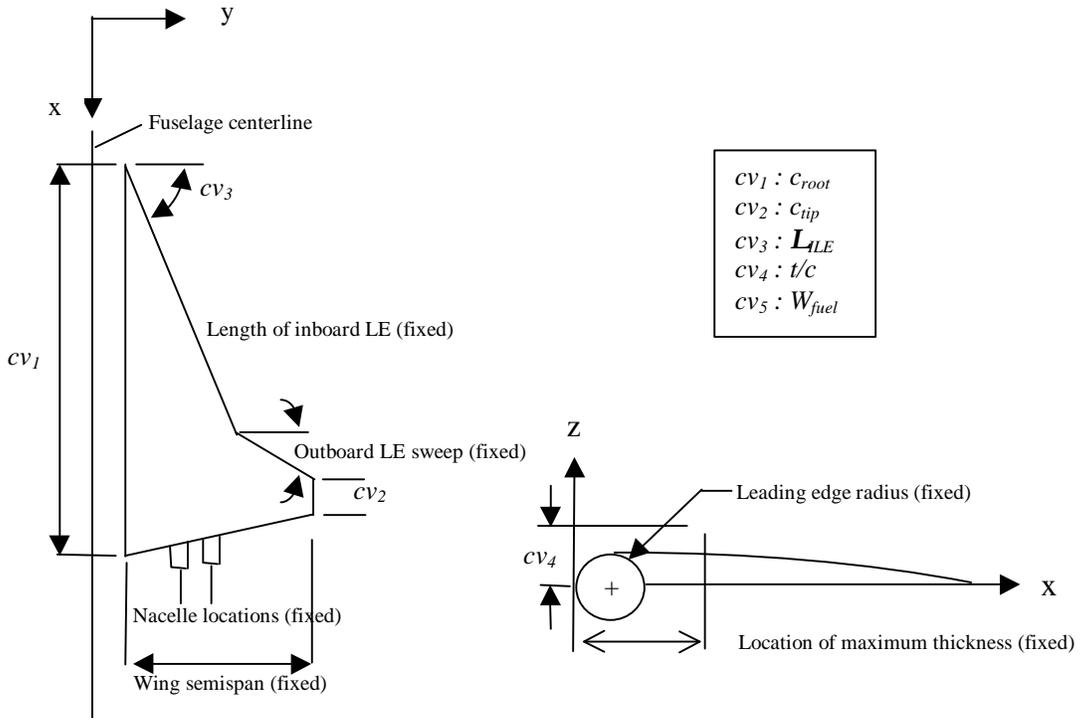
Figure 2: HSCT wing planform and 5 configuration variables
