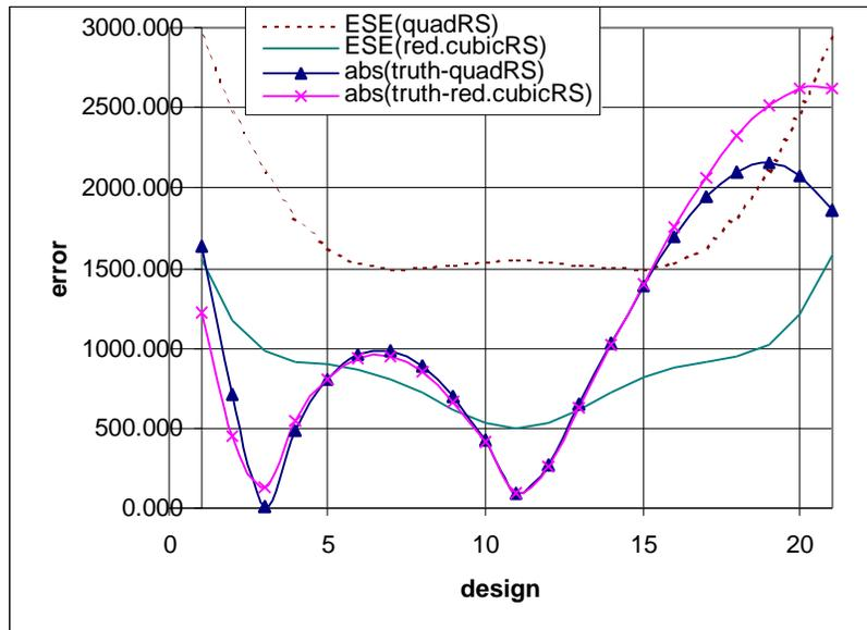
Figure 8: Estimated Standard Error (ESE) and absolute errors based on truth model for RS approximations
