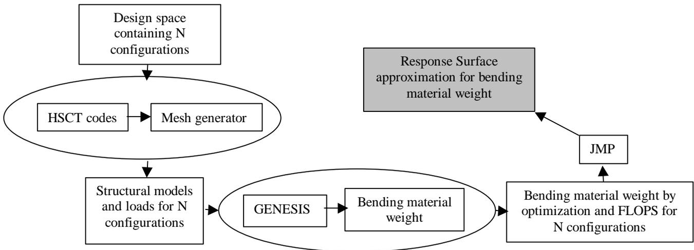
Figure 4: Flow chart for RS approximation procedure
