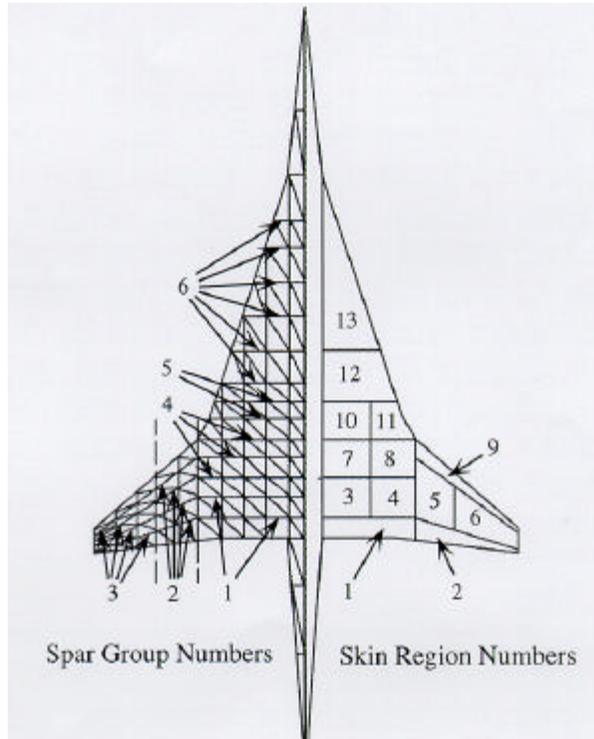
Figure 3: HSCT finite element model and structural design variables
