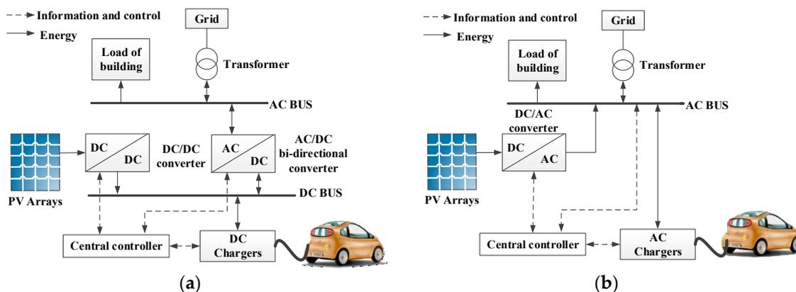
**Figure 1.** Typical structure of a PV-assisted charging station. (a) DC chargers; (b) AC chargers.
