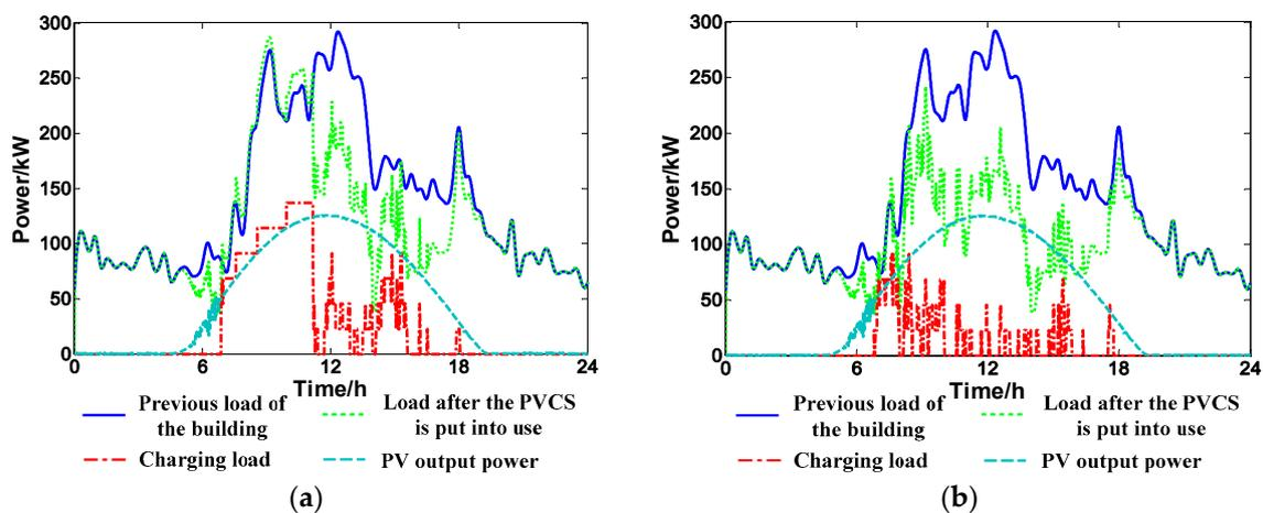
**Figure 6.** (a) Power distribution on a sunny day (scenario 1); (b) Power distribution on a sunny day (scenario 2).
