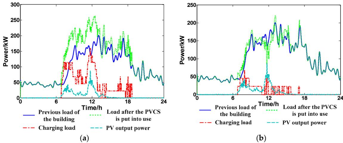
Figure 7. (a) Power distribution on a cloudy day (scenario 1); (b) Power distribution on a cloudy day (scenario 2).
