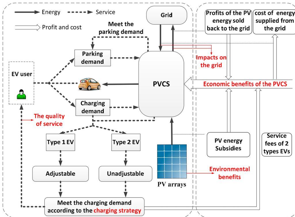
Figure 2. Typical operation mode of the office building PV-assisted charging station.
