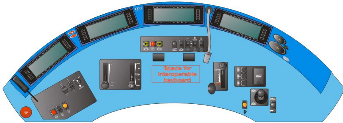
Figure 1: Standardized driver's desk as described in the UIC 612 leaflets (state on Oct.08)
