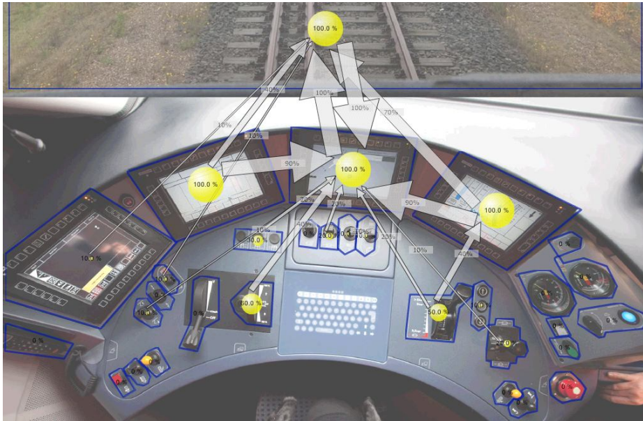
Figure 5: Star topology of the gaze transitions during braking sequence while driving with ETCS (average of all braking sequences)
