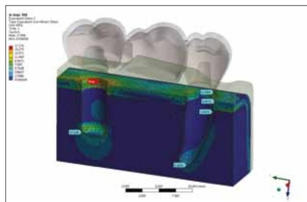
**Figure 5.** Model with non-resilient abutment and 500 N force on the implant. Maximum stress value is in the cortical bone around implant neck (17.1 MPa)
