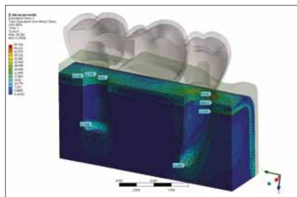
**Figure 6.** Model with non-resilient abutment and 500 N force on all three units. Maximum stress value is in the cortical bone around abutment tooth neck (49.7 MPa). High values are also recorded around the implant neck (22.8 MPa)
