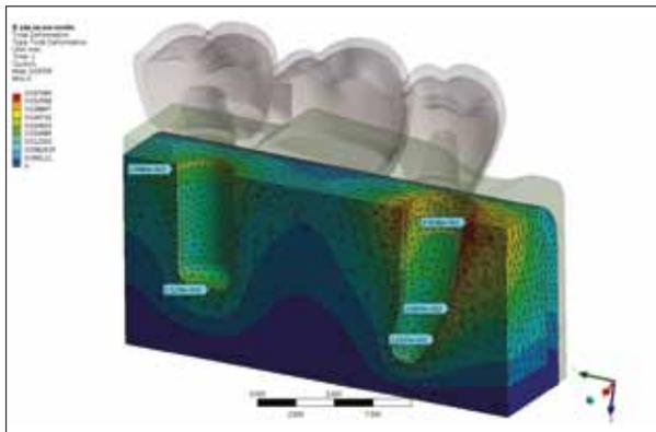
**Figure 9.** Model with non-resilient abutment and 500 N force above all three units at the same time. Maximum deformation was present in cortical bone around abutment tooth neck, mesial side (0.04 mm)
