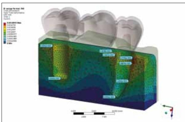
**Figure 14.** Model with resilient TSA abutment and 500 N force above the implant. Maximum deformation when the force is applied to implant is around the neck of tooth mesial side (0.001 mm)
