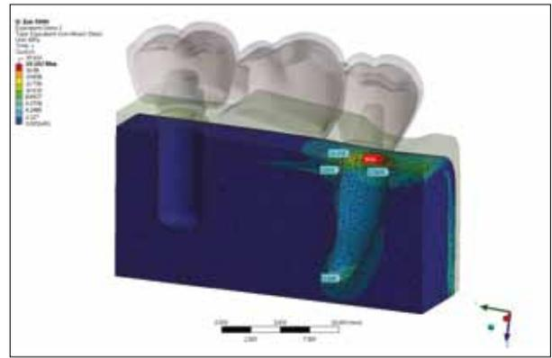
**Figure 10.** Model with resilient TSA abutment and 500 N force above the tooth. High values are recorded in the bone around the tooth neck and under the tooth root peak. Maximum recorded value is around the abutment tooth neck (19.1 MPa)
