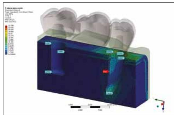
**Figure 4.** Model with non-resilient abutment and 500 N force on the tooth. Maximum stress values are recorded in the bone around the tooth neck and the middle third of the tooth root (23.7 MPa)
