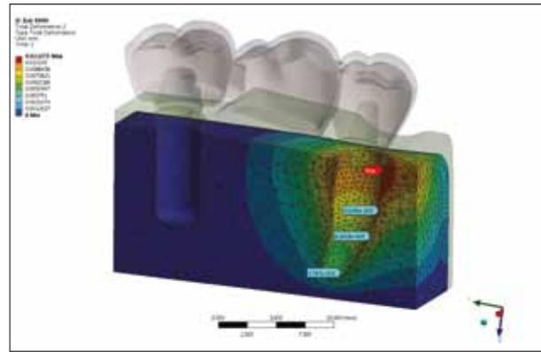
**Figure 13.** Model with resilient TSA abutment and 500 N force above the tooth. Maximum deformation values are recorded in the bone around the tooth neck, mesial side (0.01 mm)
