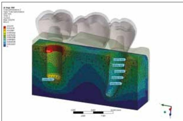
**Figure 8.** Model with non-resilient abutment and 500 N force above implant. Maximum deformation was present in cortical bone around implant neck (0.01 mm)
