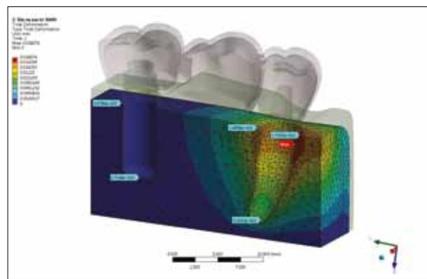
**Figure 15.** Model with resilient TSA abutment and 500 N force above all three units. The highest deformation values are also recorded around the tooth neck, mesial side (0.02 mm)
