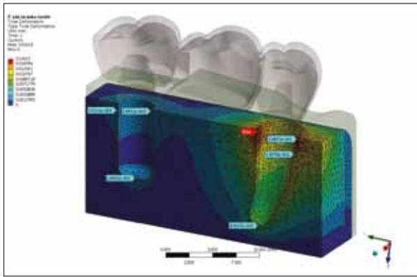
**Figure 7.** Model with non-resilient abutment and 500 N force above natural tooth. Maximum deformation was present in cortical bone around abutment tooth neck (0.02 mm)
