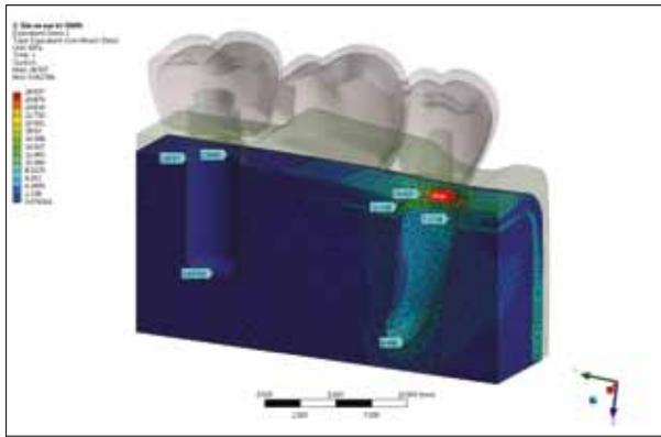
**Figure 12.** Model with resilient TSA abutment and 500 N force above all three FPD units. The highest stress is also in the bone around abutment tooth neck (28.9 MPa)
