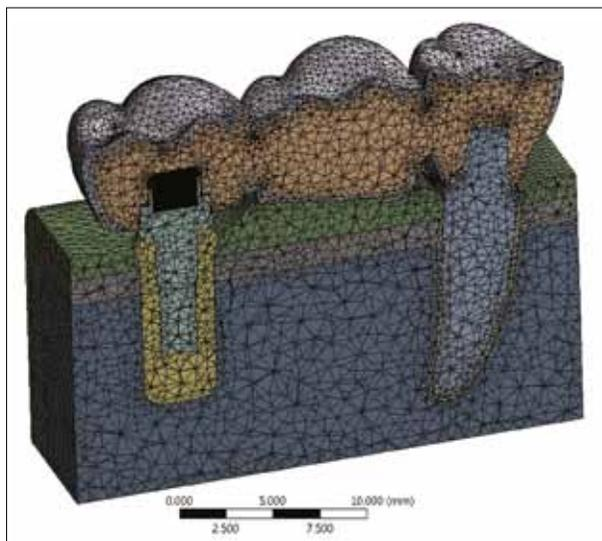
**Figure 3.** Network of elements and knots of the tooth-implant supported FPD
